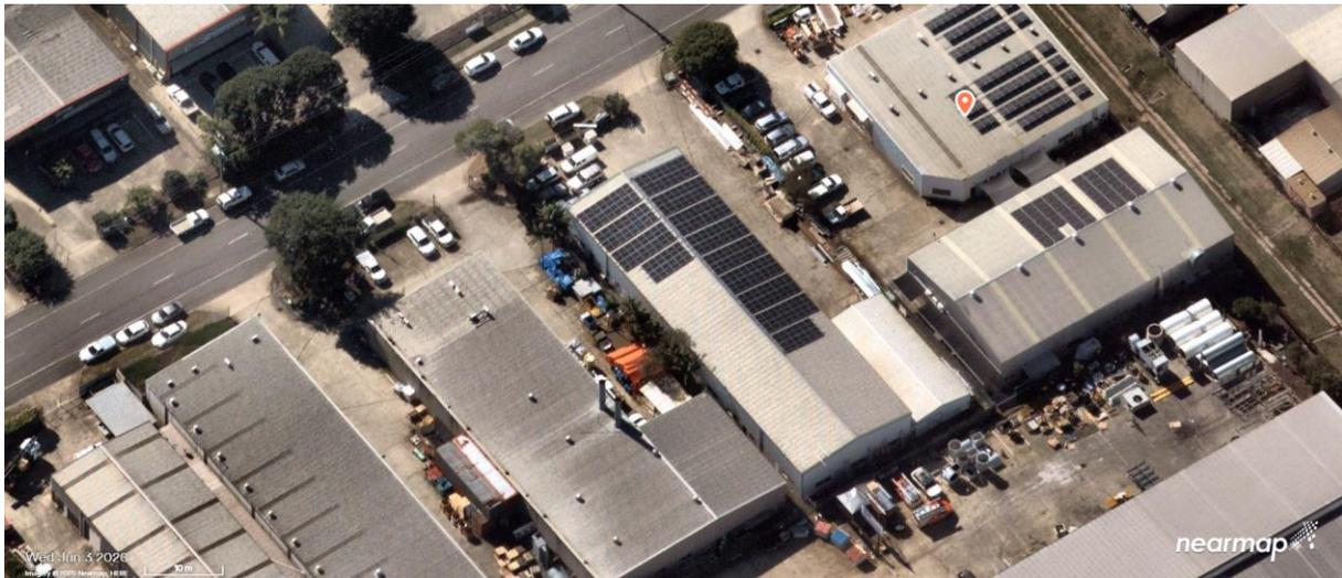
In June 2020, DS Energy delivered a 66kW installation utilising 200 330W Phono Panels and the Fimer 50kW Inverter.
